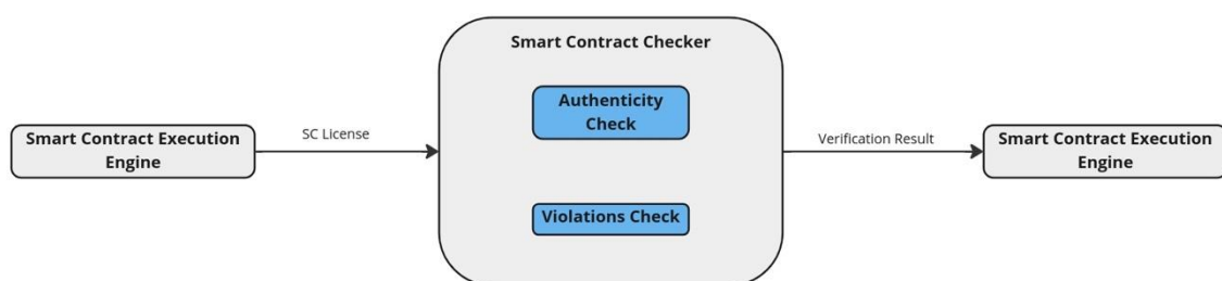
Figure 23: Smart Contract Checker High-level Architecture
